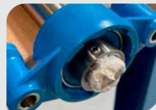
3) Remove any large lumps of grease
