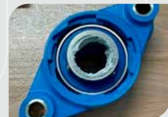
1) Lubricate the inside of the inner ring
