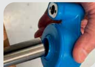
2) Insert the bearing house over the shaft
