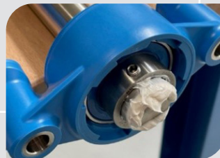
3) Remove any large lumps of grease
