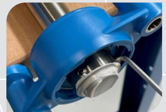
4) Tighten set screws
