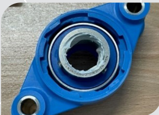
1) Lubricate the inside of the inner ring
