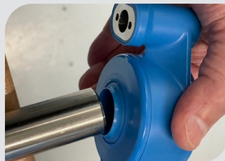
2) Insert the bearing house over the shaft
